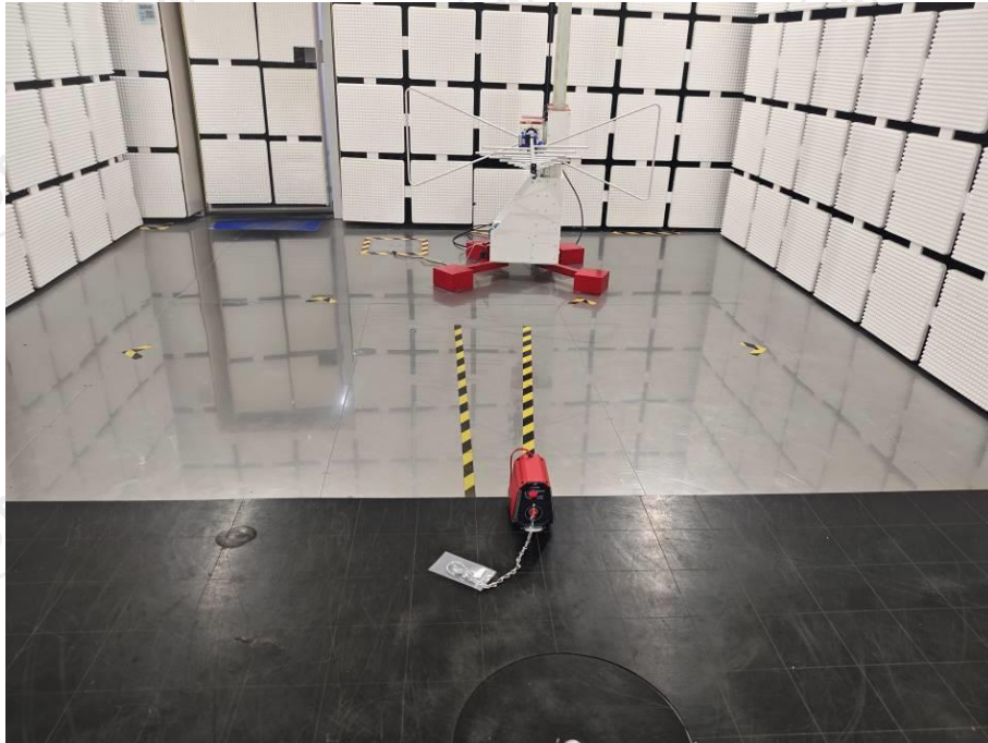
Radiated emission (30 MHz to 1 GHz) Test View
